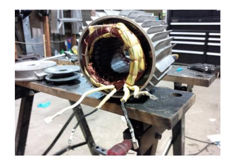
If after testing, the motor winding insulation has deteriorated to a level below the motor manufacturers defined limits, the recommendation is to purchase a complete fan, manufactured and certified in accordance with latest version of the EN 12101-3 standard.
